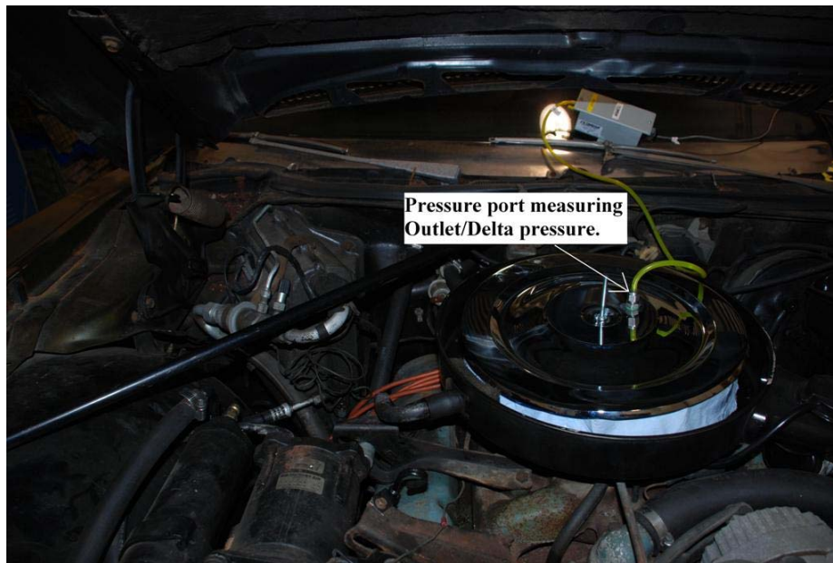
Fig. 3.12. Pressure port location for 1972 Pontiac Grandville.
