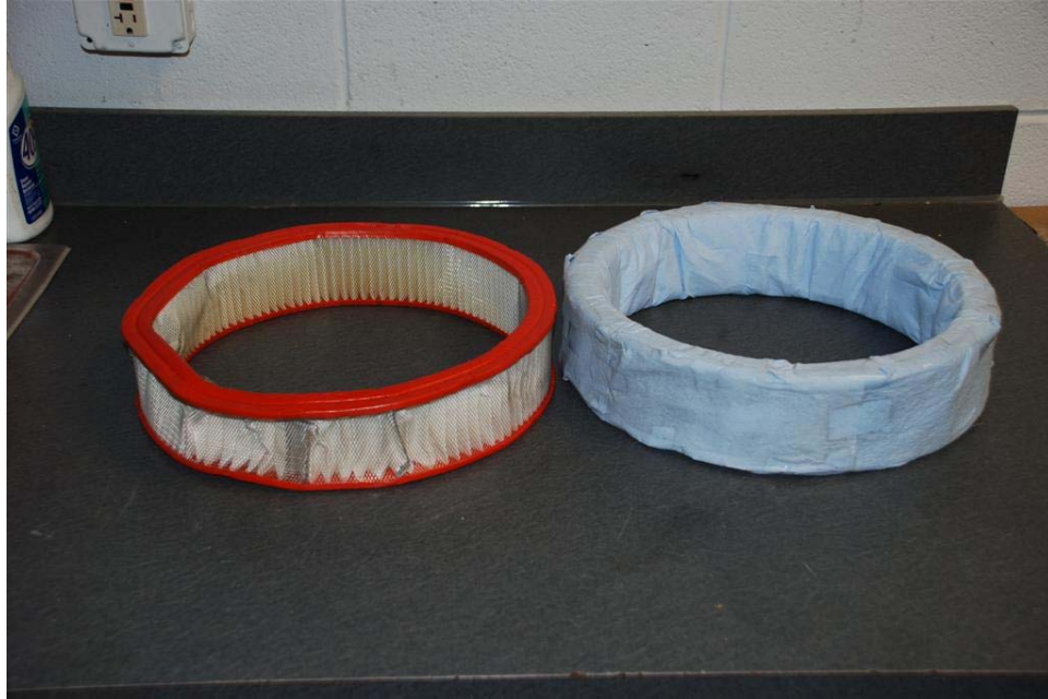
Fig. 2.5. 1972 Pontiac Grandville air filter. Filter on the left shows damage that occurred during “severely clogged” filter testing (see Sect. 3.3.1).
