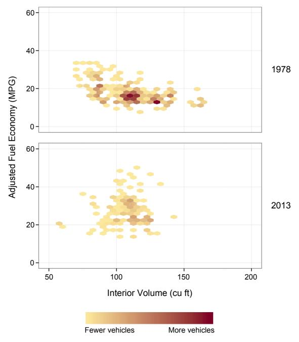
The data in Figure 3.2 illustrate the "compression" in the range of interior volumes for car type vehicles since 1978. In MY 1978, there were mainstream car type vehicles on the market with interior volumes ranging from about 70 cubic feet to about 160 cubic feet, with a large number of offerings at both ends of the spectrum. Today, mainstream offerings
