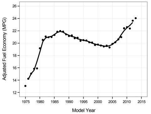
These two figures show that fleetwide adjusted  $CO_2$  emissions and fuel economy have undergone four clearly defined phases since 1975. Figure 2.3 shows fleetwide adjusted fuel economy, weight, and horsepower data for MY 1975-2013 from Table 2.1. All of the data in Figure 2.3 are presented as percentage changes since 1975. Vehicle weight and horsepower are critical vehicle attributes in that higher values, other things being equal, will increase  $CO_2$  emissions and decrease fuel economy.
